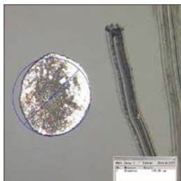
Before etching: Tin residue Ø 180 µm on the air side
